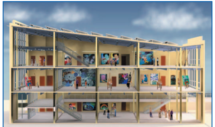
Artists for Humanity is a non-profit organization that offers paid apprenticeship programs in the arts to inner-city teens. AfH was awarded a $20,000 grant for a feasibility study and later a $500,000 grant for design and construction of its 45-kilowatt producing roof-mounted PV cells, and glass curtain wall. © T.R. White
